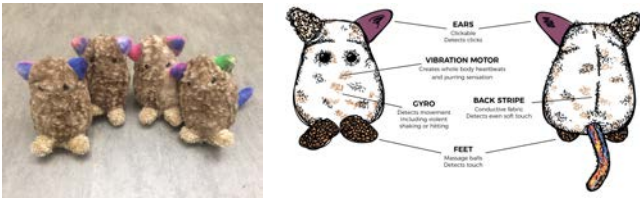
Figure 1. (a) The technology probe design; (b) Overview of the interactive components in the technology probe
