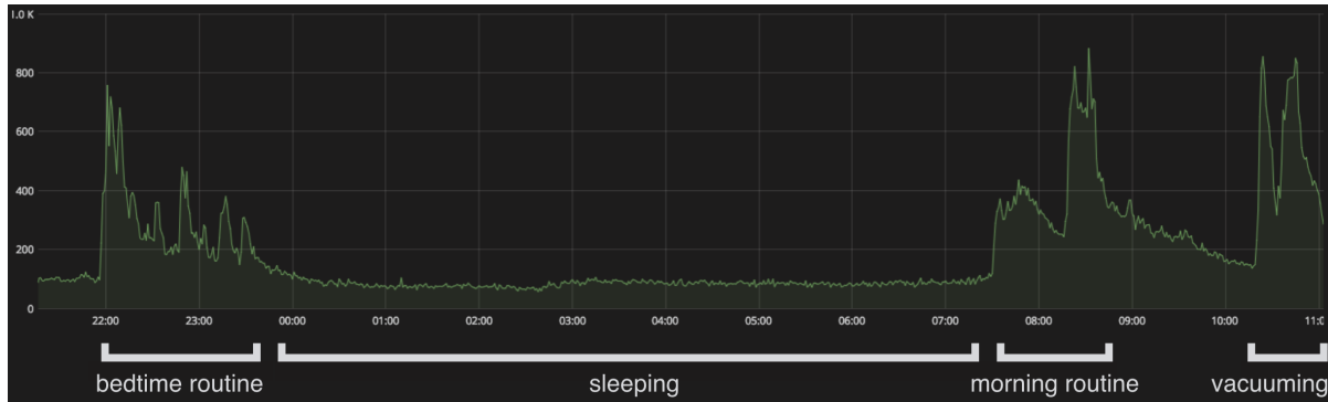
Fig. 1. P2 daily routine captured by air quality monitors
